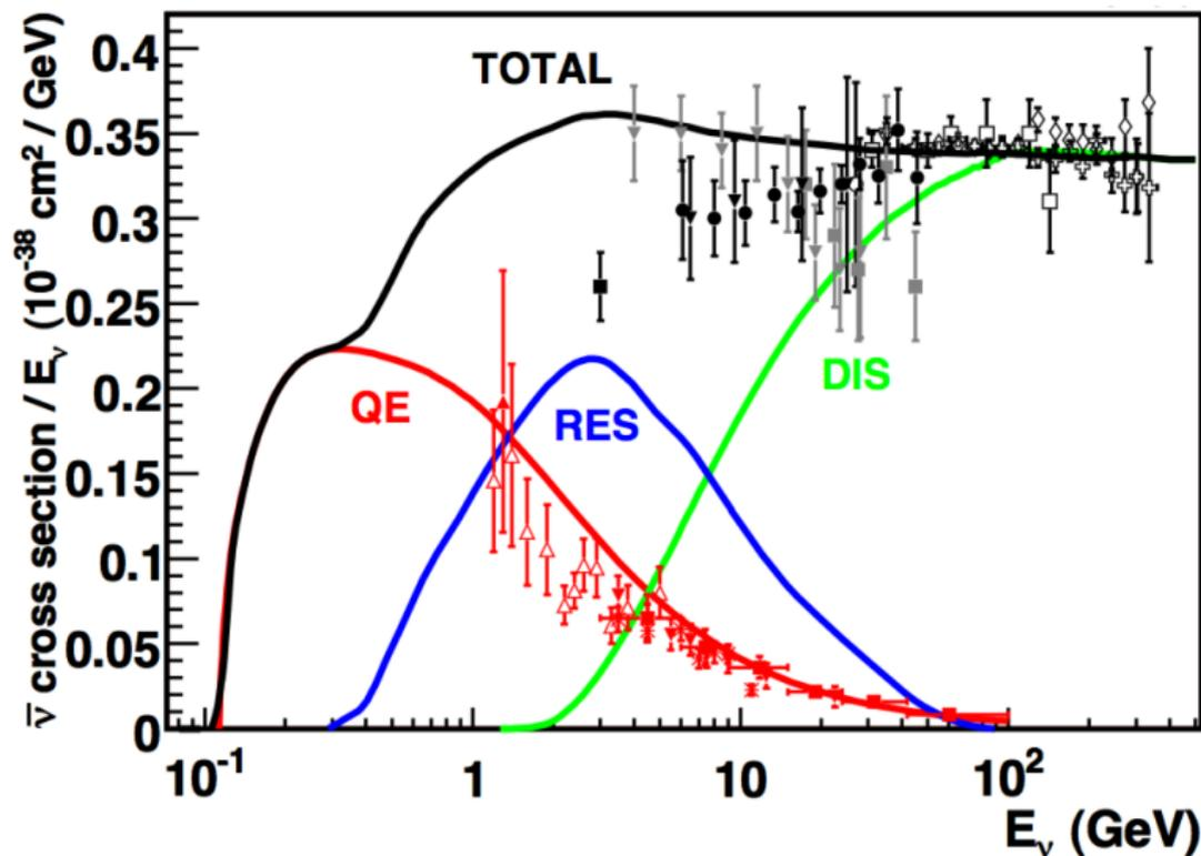
Cross section in a detector: various processes
